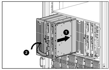
Figure 1-29: Installing a server blade
